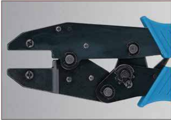
RG-9317 FOR COAX CONNECTORS RG-58, 59, 62 AU BNC & TNC
