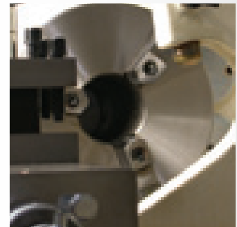
LARGE 3-1/8" SPINDLE BORE
