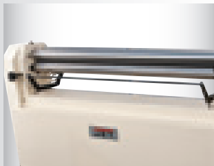
SAFETY BAR, WHEN PUSHED WILL SHUT DOWN THE MACHINE.
