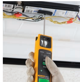
Easily determine if ballast is working.
