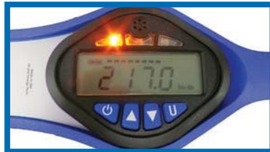
The yellow LED illuminates within 10% of target torque.
